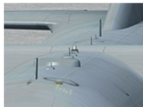
Modified Oil Cooler Flaps
