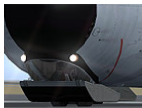
APU Exhaust Heat- Protection
