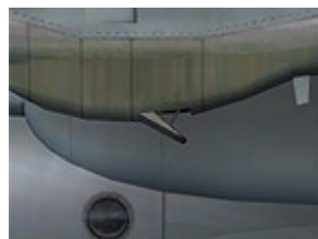
Modified Oil Cooler Flaps
