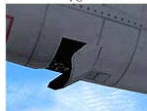
Engine Oil cooler flaps(4) VC
